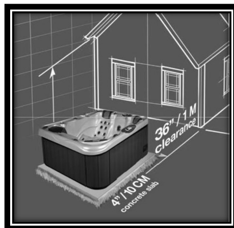
Figure 1 - Space Required (Clearance) and Support
